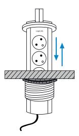
Tighten the detachable locking ring clockwise from the bottom of the socket.
