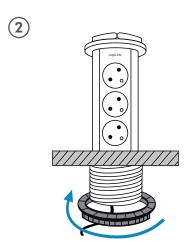
Remove the detachable locking ring from the socket, and put the socket into the hole.
